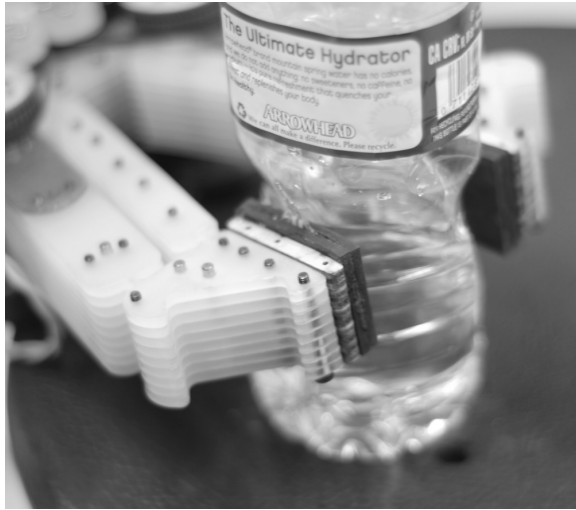
Figure 1: Unstructured manipulation tasks envisioned to be performed by service robots include door-opening and grasping common household objects. Pictured here only to illustrate that many such tasks can tolerate errors of a few millimeters, provided some measure of compliance exists in the mechanism or its control scheme.
