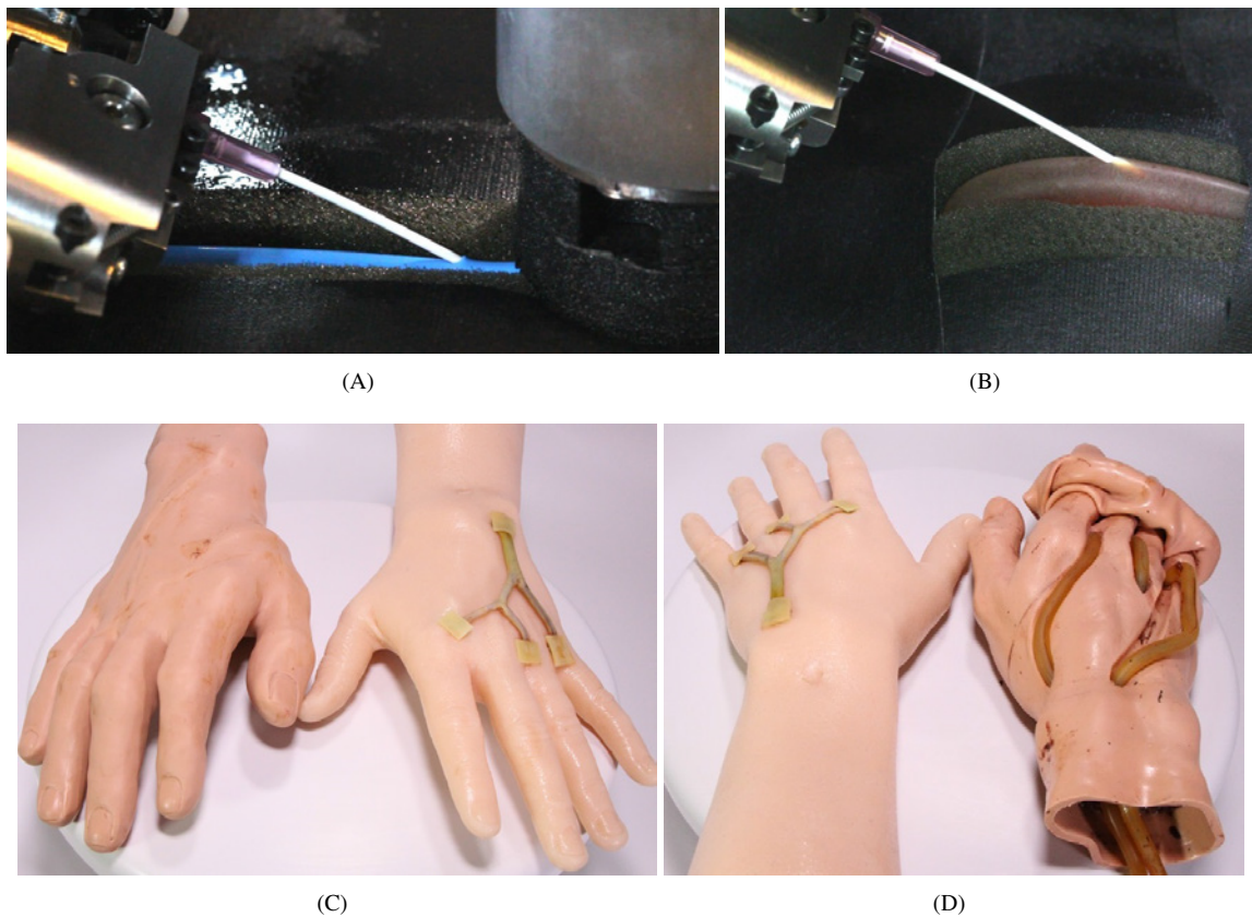
Figure 6.2: Commercial Off-The-Shelf IV Phantoms. A: Twister (“balloon-animal”) 160Q-size balloon. B: Latex tubing. C-D: Simulaids IV Hand Simulator 147R next to our custom phantom.
