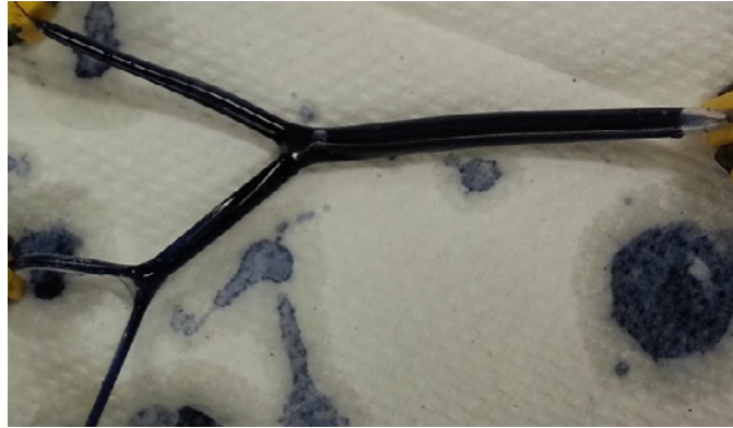
Figure 6.3: Silicone Venous Network Patterned On Author’s Anatomy. Although we were able to fabricate the venous network in silicone, the force “pop” was not close enough to that of a real vein.
