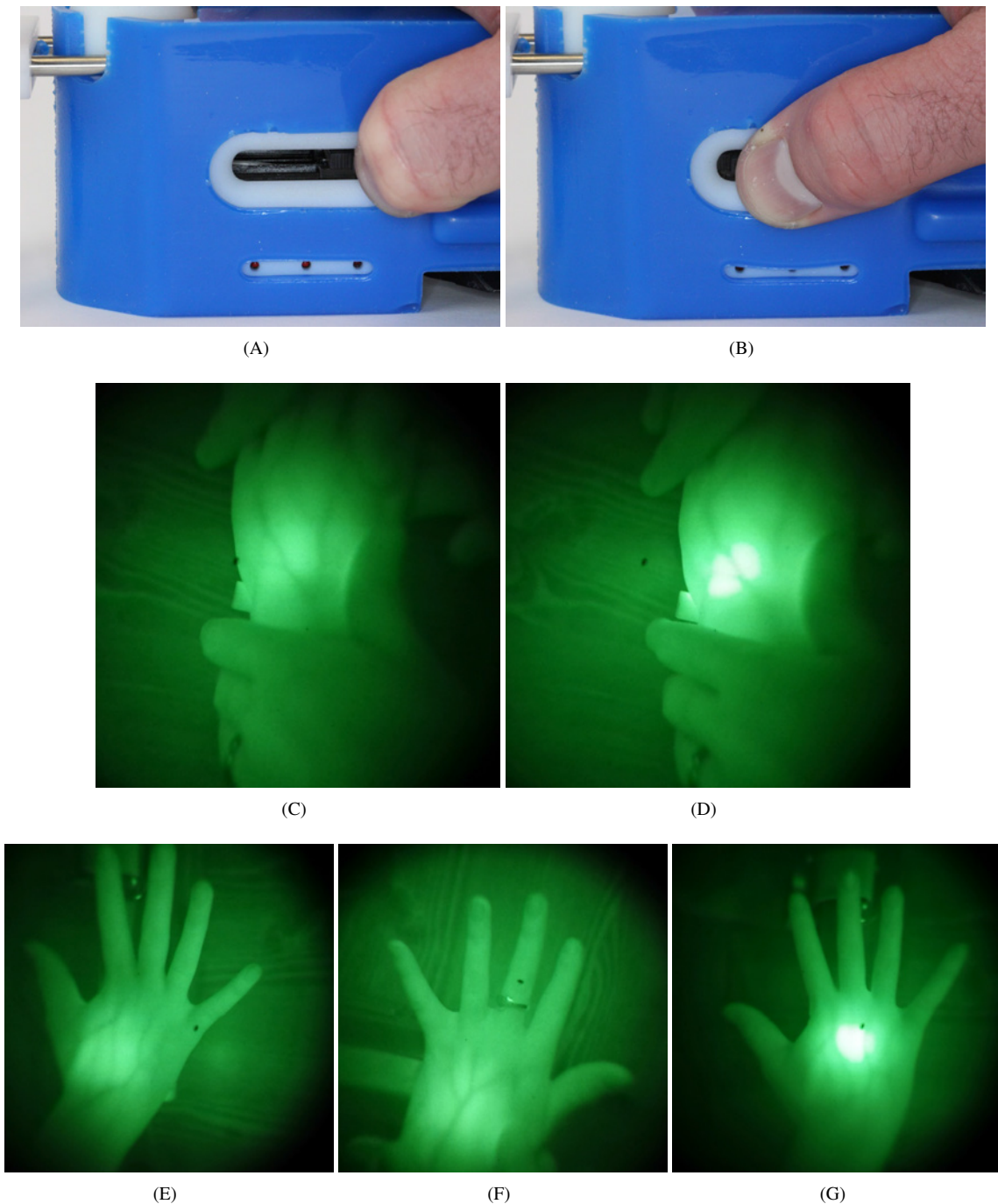
Figure 5.5: eye.Vease, Laser Brightness Control. We included a method of controlling the laser's brightness because different patients and regions within the same hand require different amounts of light to show the veins properly. A-B: Brightness control slider/thumb-adjustment-bar. C-F: Images recorded by holding a smartphone's camera to the NIR-goggles' eyepiece. The in-person view is much superior. C-D: 5-year-old, Caucasian male. E-G: 7-year-old, Caucasian female. D, G: Excessive laser brightness causes saturation/pixel-blooming in the NIR-goggles, thereby hiding the veins. C, E, and F: A lower laser brightness allows us to see the veins.
